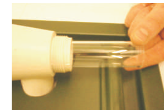
7). Carefully remove quartz sleeve
