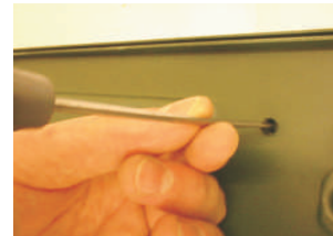
3). Remove Plastic Fixing Rivets.
