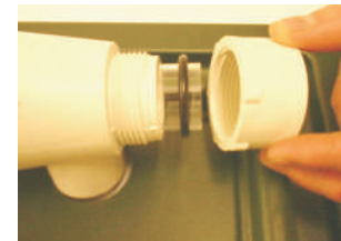
6). Unscrew end caps and remove o rings, (We recommend that you replace these annually)
