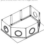
Now using the leg cross brace bars (parts 20 & 21) and 14 of the remaining plastic keys (part 2) insert them one at a time, working your panel empty. Lock the plastic keys by quarte turning them, using the provided tool (part 1).
