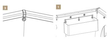
Place the Inpond 5 in 1 filter inside the pond and thread the cable between the liner bag (part 5) and the frame of the pool. Use the section of liner that you left unattached in step 15, this will help to keep the cable tidy and out of harms way. Once the cable has been threaded through the gap, attach the eyelets on the liner bag to the holes on the top rail using 2 of the Plant basket fixing pins (part 3). See Inpond instructions on how to set up the filter correctly. Do not turn the Inpond
