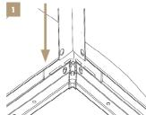
Your Affinity Pool should now have all 8 of the leas inserted the right way up and be ready to have the plastic keys (part 2) inserted at the bottom of the top rails. It should look like the image below with all 8 legs inserted.
