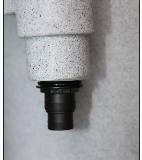
STEP 3: Ensure the hosetail is hand tightened until the rubber O-ring seals on the inlet face. (DO NOT OVERTIGHTEN)
