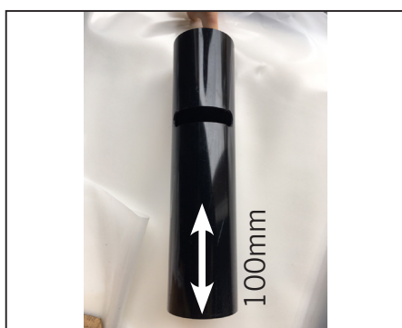
16. Take the black pipe you removed in step 12 in preparation for cutting a 100mm slit in it.
