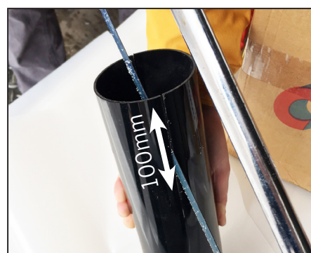
17. Use a saw to make a 100mm slit in the black pipe on one side of the pipe only. This is now your cleaning pipe.
